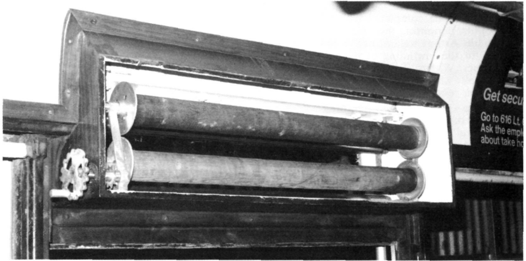
View of the newly constructed side destination mechanism during trial fitting.
