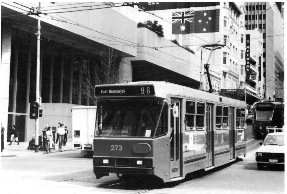
Pantographs on Bourke Street. A2 class 273 crosses Elizabeth Street enroute to East Brunswick on 17 September 1987. Route 76 has been converted to pantograph operation for the through LRV service from St Kilda and Port Melbourne.
