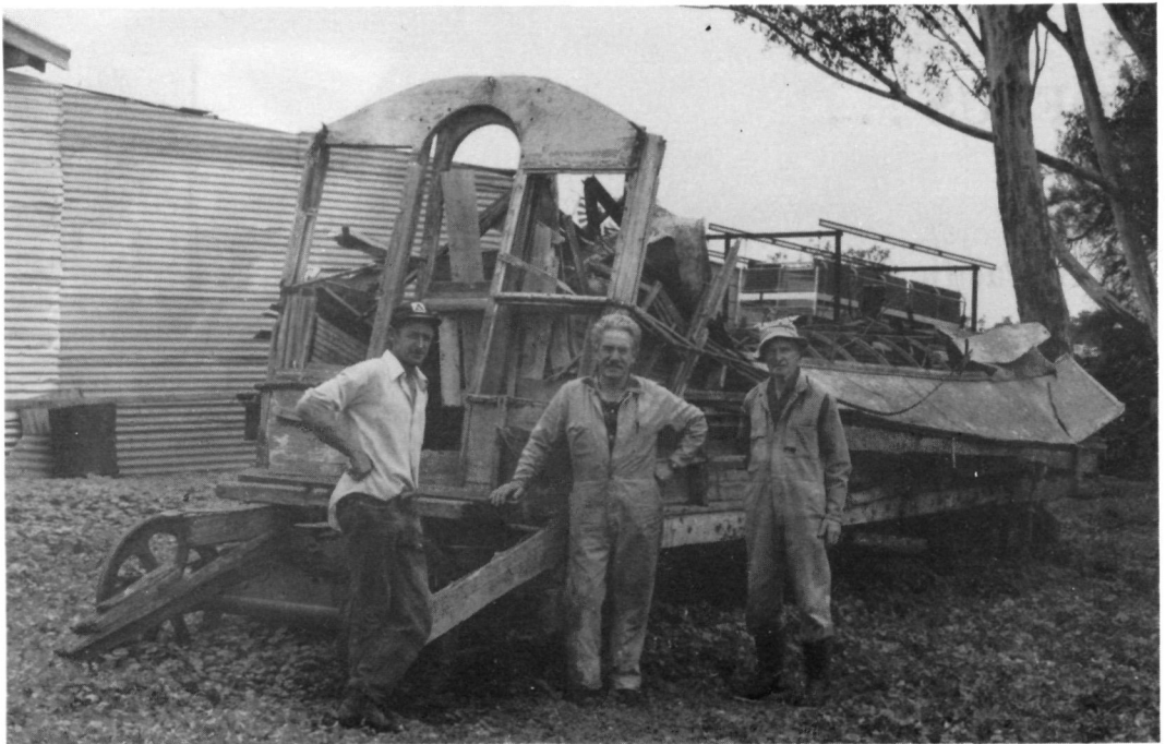
This photo of Bendigo bogie steam trailer No. 2 (formerly single truck battery car No. 3) was taken on 19 April 1989. It had been on the property of an Elmore farmer for some sixty years.
