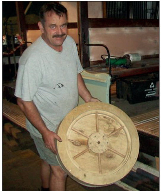
Craig Connelly proudly displays the wooden pattern for the casting of wheels for the eventual manufacture of bogies for the double-deck car.
