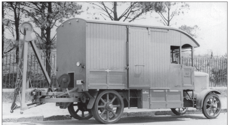
The Karrier in its original tramway recovery configuration in 1928. STM archives
