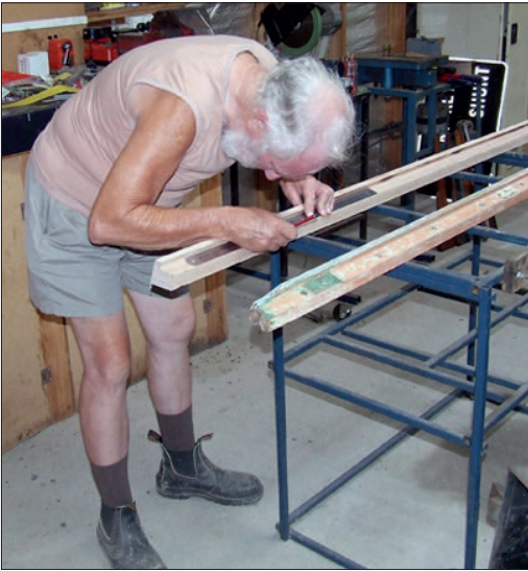
John Withers marks out positions on one of the door jambs for SW5 849 where the hinges will be chiselled in.
