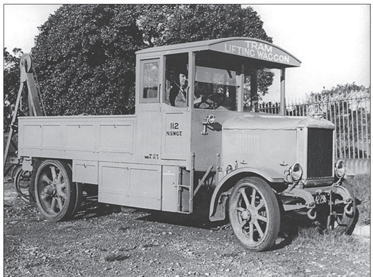
The Karrier Tram Lifting Wagon shows its rebuilt body style in 1936.
