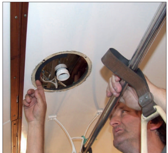
One of the polished stainless reflectors is re-installed back into SW5 849 by Anthony Smith before the frosted glass cover is reinstalled over the light.
