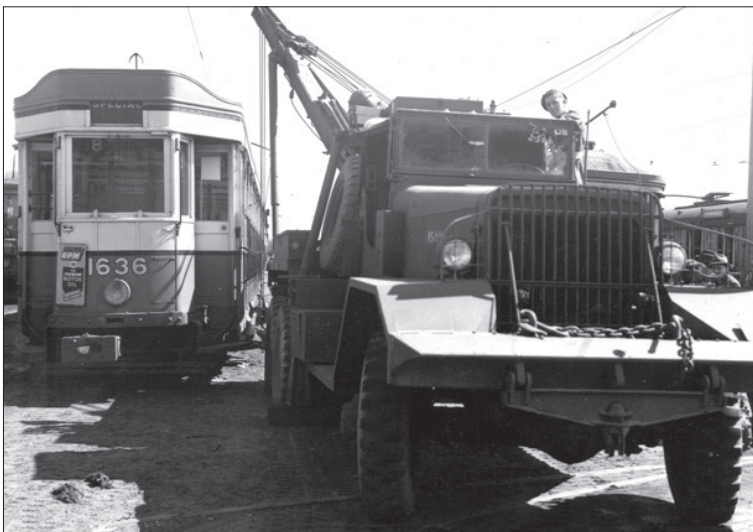
The Kenworth's lifting ability was tested at Randwick Workshops in 1946 using P car 1636.
