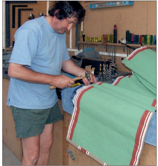
Anthony Smith carries out the 'riveting' (pardon the pun) task of securing the storm curtain runners to the canvas curtains with copper rivets.
