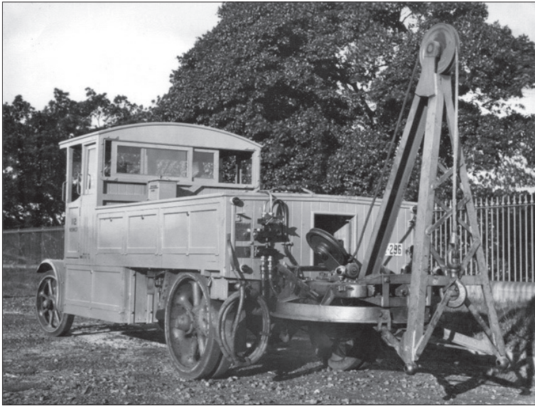
A rear view of the Karrier (carrying departmental number 112) in its final form showing its lifting gear. STM archives
