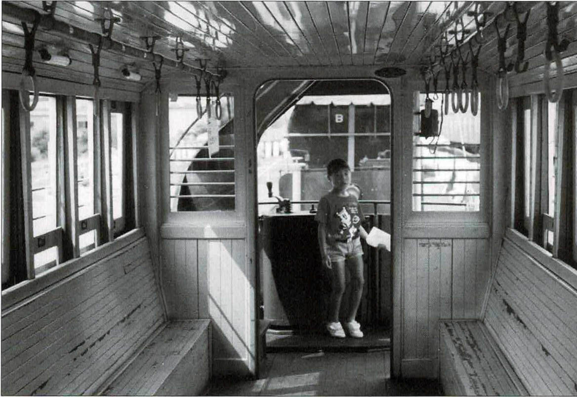
An interior view of No. 5 which is probably the original interior of car 720, unchanged but for a new ceiling. Note the very narrow seating provided. JUNYA YAMACHI
