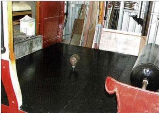
The air inlet filter and the air reservoir are the only easily visible parts of the air system since the laying of new flooring in the drop ends of tram 15.
