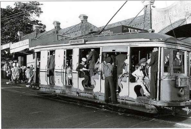
K 1295 prepares to depart Neutral Bay Wharf with a standing load of passengers, in about 1954. The car is overdue for an overhaul, as evidenced by the rotten bow rail.
