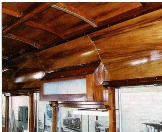
An interior view of the ceiling panelling in the drop-centre section of W3 663, showing the impressive varnished timbers. Anthony Smith
