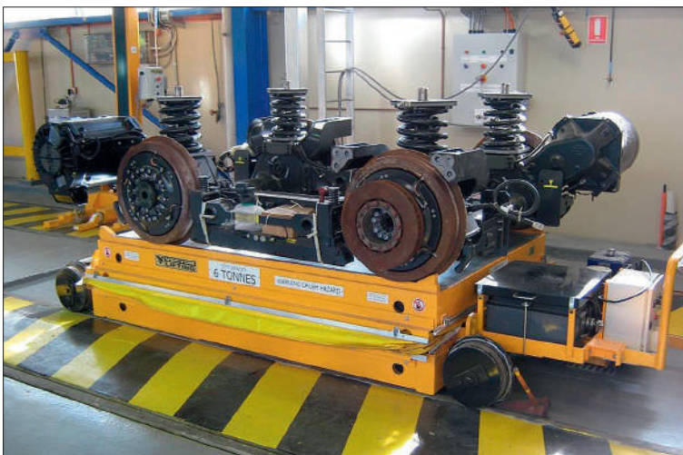
The bogie drop trolley being tested in February 2011.
