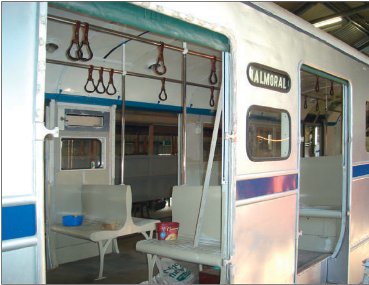
Newly installed grabrails, strap hangers and side destination boxes in FM 400.
