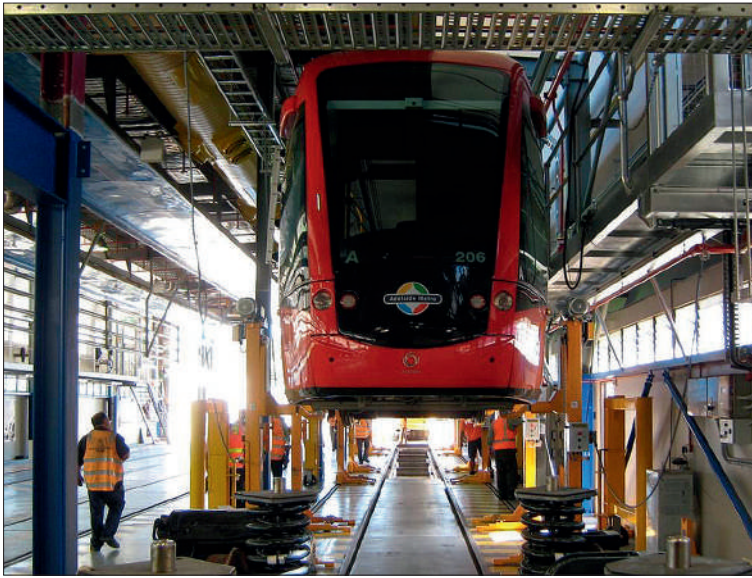
Citadis tram 206 is raised on Road 3 North for a lifting test in February 2011.
