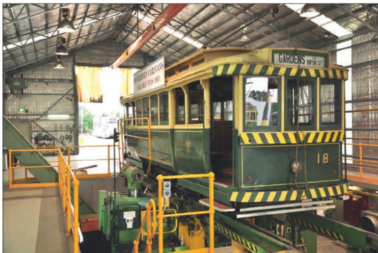
No. 18 on the wheel lathe at Preston Workshops on 16 October. Alastair Reither
