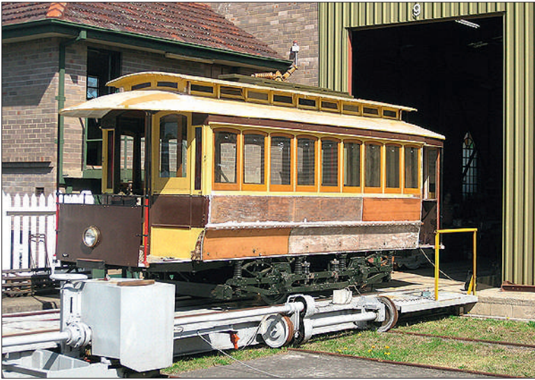
C car 37 was placed on its refurbished Peckham truck on 26 September and driven onto the traverser for photographs. Mick Duncan
