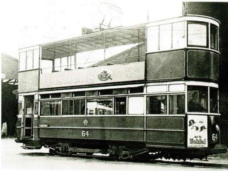
Car 64, the latest design, with partially enclosed upper deck.
