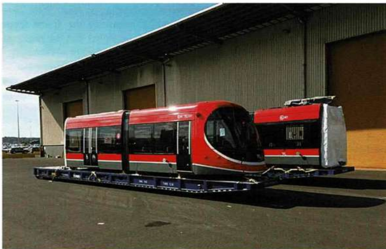
A Canberra car on the wharf at Port Kembla on 3 May 2018. The cars are unloaded at Port Kembla and trucked to Canberra in two sections.
