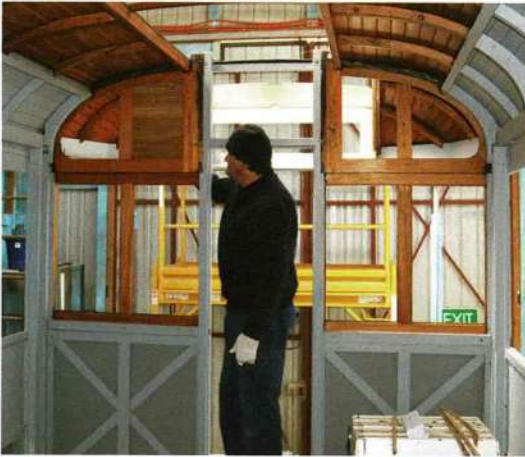
New blackwood panel being trial-fitted to the driver's bulkhead of 792. Jacqui Smith
