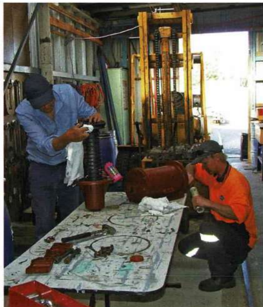
Frank Schroeders and Anthony Smith reassemble the brake cylinder for 792. Jacqui Smith
