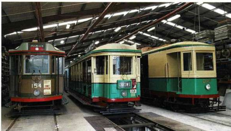
A running shed view showing LP class 154, O class 1111 and freight car 24s. Additional pit boards have been placed over the pit in front of 1111 to make it easier to attend to the trolley pole. Scott Curnow
