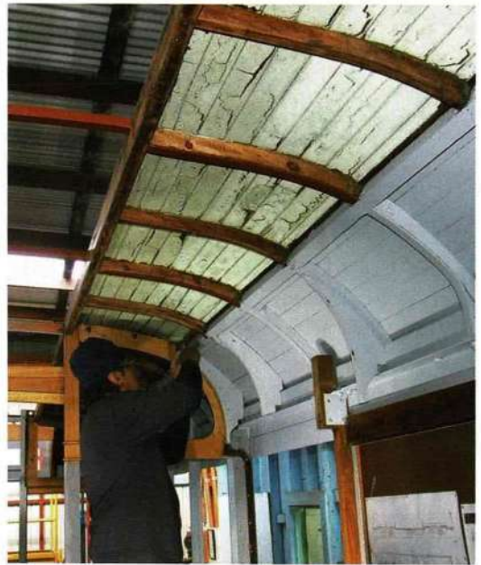
Anthony Smith removing old colorflek from the drop-centre ceiling boards on 792. Jacqui Smith
