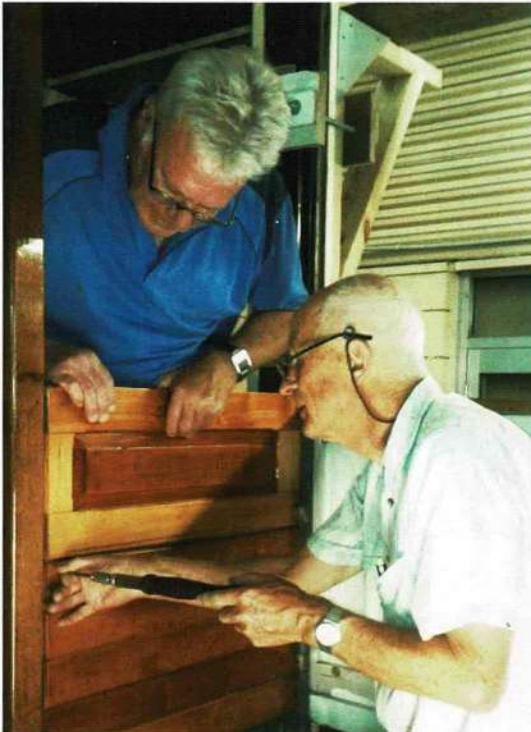
Graham Wright and Rob Hodge refitting Huon Pine interior panelling to the saloon of tram 14. John Binns
