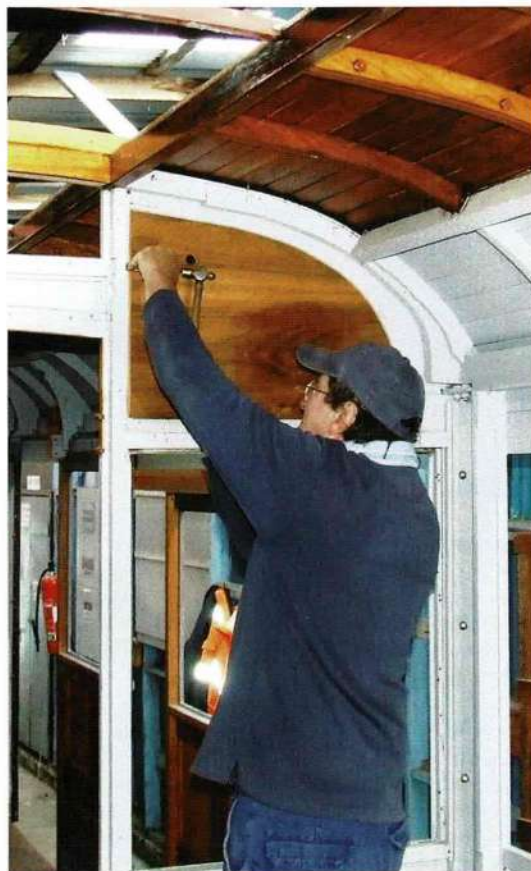
Anthony Smith fitting new ply panels to the drop centre bulkhead of 792.
