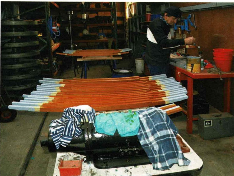
The new vent roof ribs being prepared for fitting to 792.
