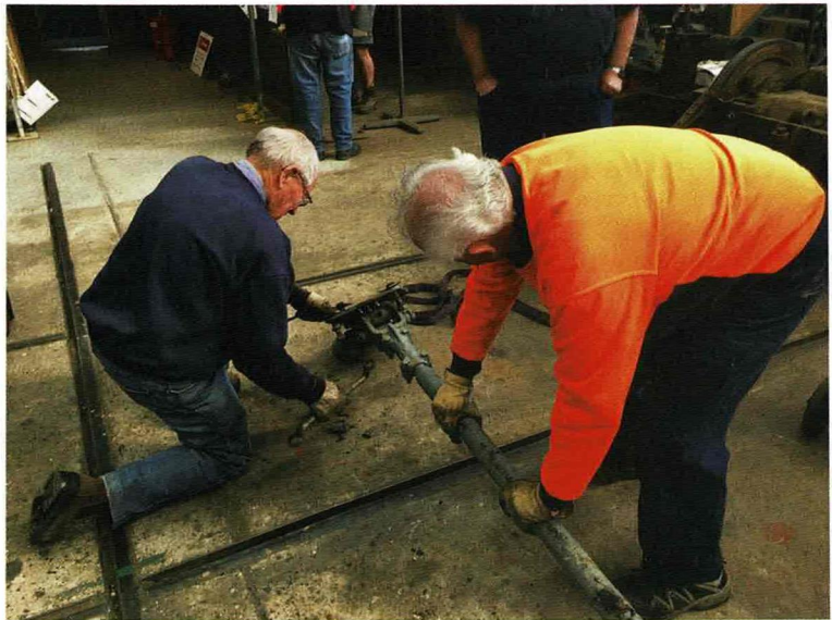
Bill Parkinson and Mal Macaulay separate the trolleybase and pole from car 11. Michael Hatton
