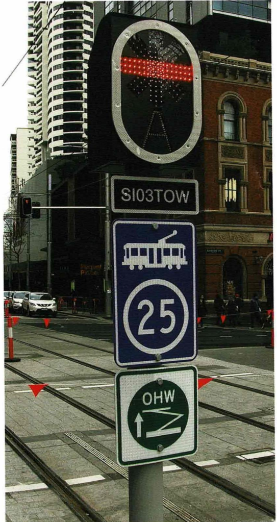
A Sydney CBD and SE light rail sign in George Street at Town Hall. This location is the transfer point from the Aesthetic Power Supply (APS), known as third rail, from Circular Quay to Town Hall, and the Overhead Supply System used for the rest of the light rail lines. R.I. Merchant
