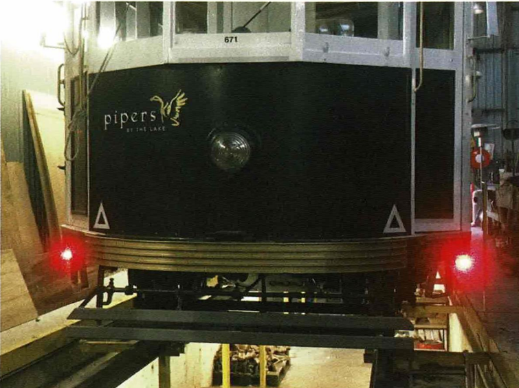
W4 671 has been fitted with red and white auxiliary lighting. Neville Britain
