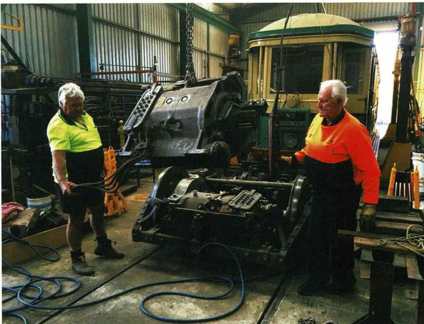
The museum's overhead cranes make light work of removing a motor from one of 141s's bogies. Michael Hatton
