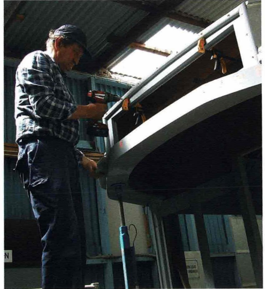
Anthony Smith fitting new 'D' mould cover strips to the front destination fascia of 792. Daniel Edwards
