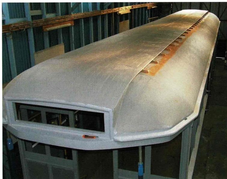
View showing roof of 792 after final covering.
