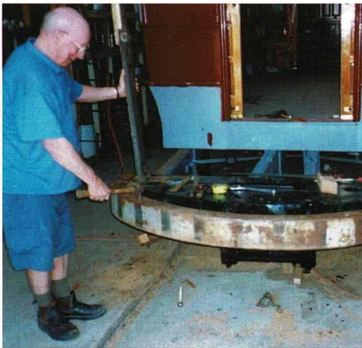
Peter Letheby doing a test fit of 118's bumper on the rebuilt platform during its restoration prior to its launch in May 2010.
