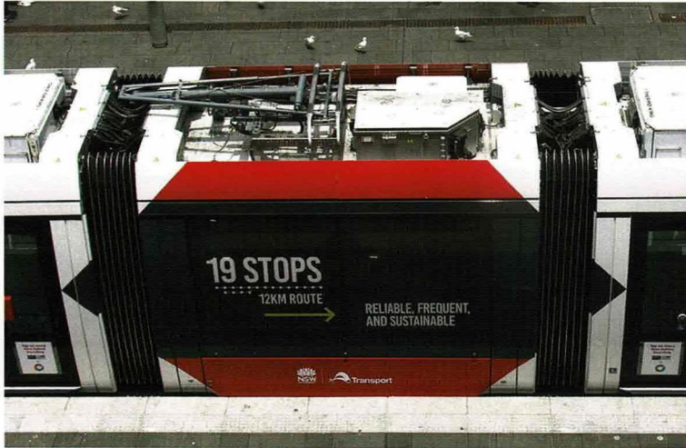
The pantograph folded down on the top of Citadis X05 car 17 at Circular Quay.
