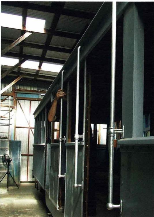
Restored handrails being fitted to the drop-centre of 792. Jacqui Smith
