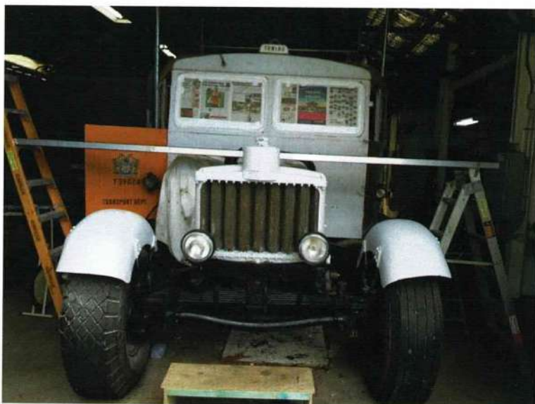
Restoration work on the Scammell showing the first layers of undercoat paint.
