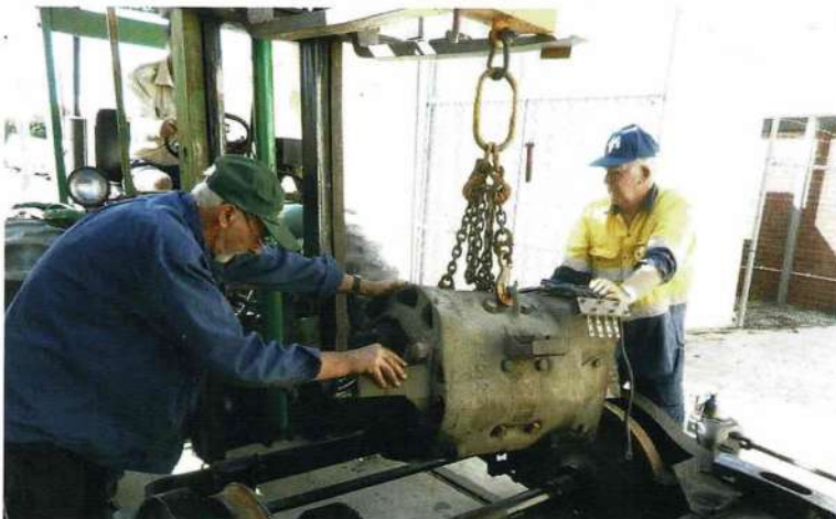
Graham Barkla and John Barlow guiding the removal of a motor from a Melbourne No.15 truck on 11 March.
