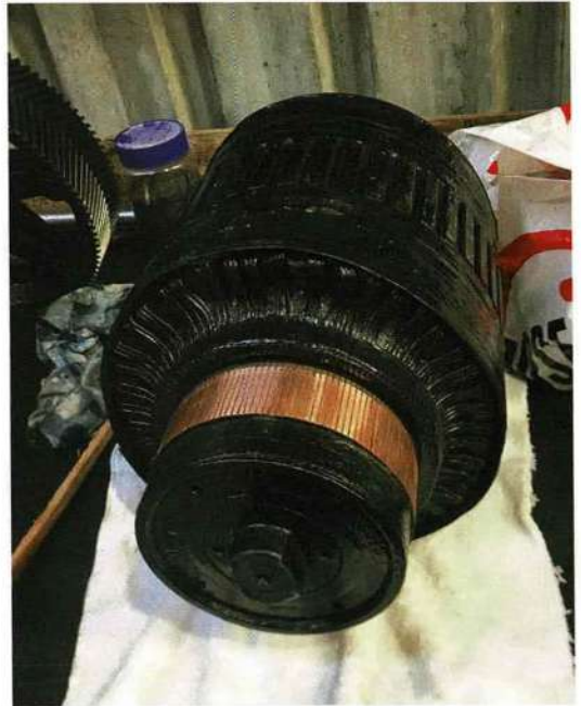
A good-looking overhauled armature of a DH 16 compressor. Paul Mong
