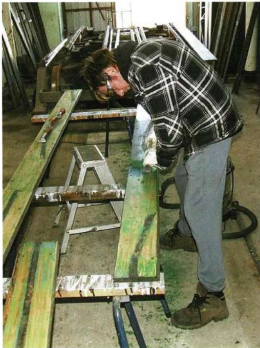
Daniel Edwards scraping old paint and varnish from a saloon wall board from 826. Jacqui Smith
