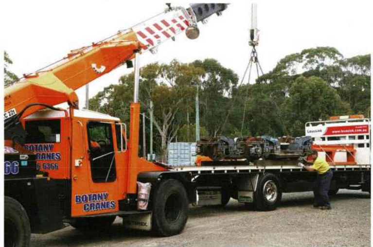
Loading the spare motorised bogie from 2106 for movement to Leusink on 30 September. Martin Pinches
