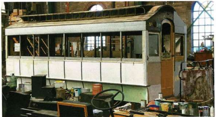
The western side of Melbourne cable trailer 589 showing the restored side panels. David Critchley
