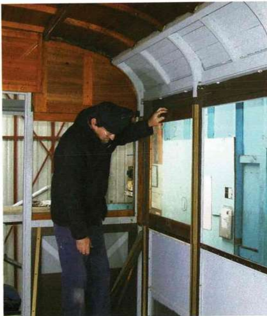
Anthony Smith trial fitting a saloon widow sash to a window pocket on W5 792. Jacqui Smith
