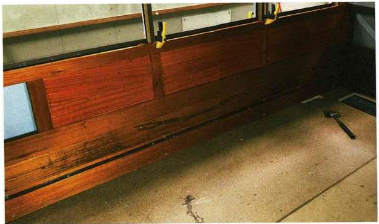
Anthony Smith trial fitting a saloon widow sash to a window pocket on W5 792. Jacqui Smith
