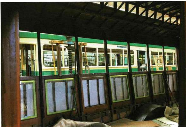
The western side of Melbourne cable trailer 589 showing the restored side panels. David Critchley
