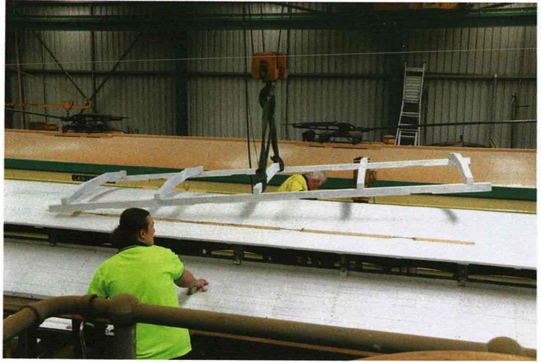
The trolley bridge from D 117 is being removed. Martin Pinches
