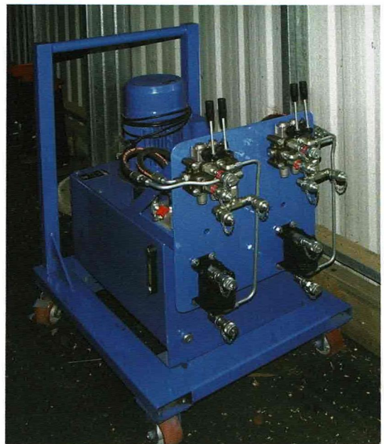
New control unit for hydraulic tram lifting equipment.
