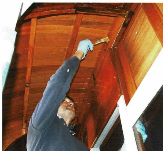
The No 2 cab ceiling of 792 receiving its first coat of clear lacquer. Jacqui Smith
