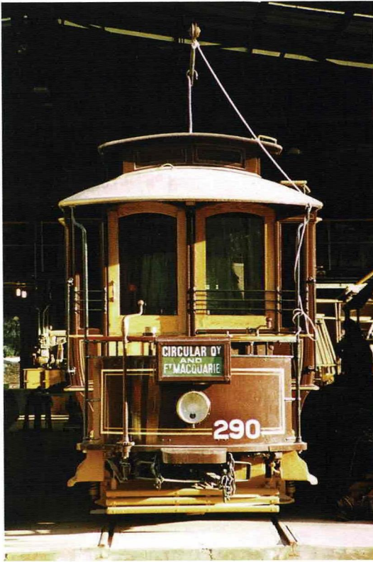
The narrow width of the C cars, 2.04 metres, is apparent of this view of 290 in the doorway of the workshop at Loftus. Dale Budd
