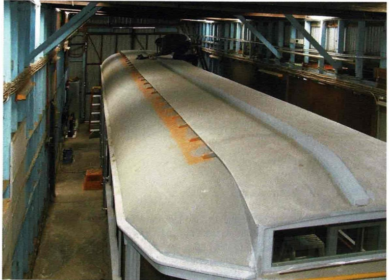
Anthony Smith fitting the roof mounted cable duct on 792. Jacqui Smith
